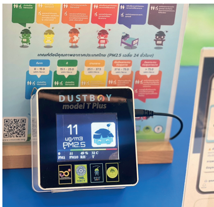
A device that measures small particulate matter in the air using sensor technology (DustBoy).
